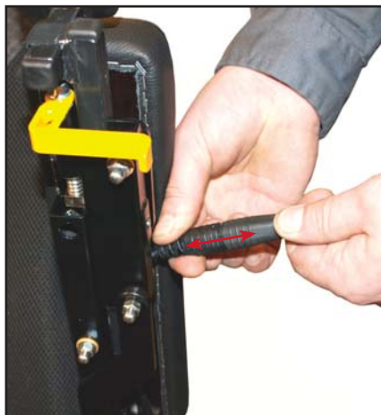
Unplug the joystick. Mount a new joystick in reverse order.
