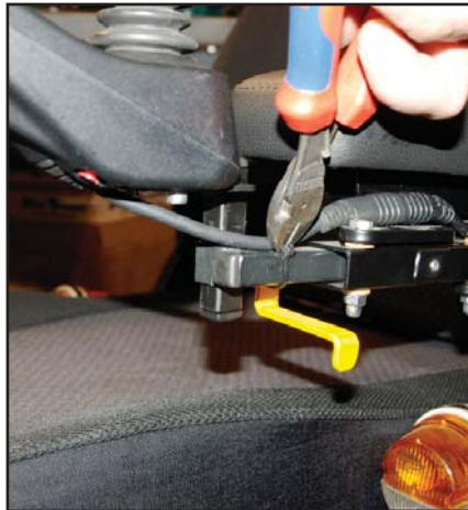
Remove the plastic strip that keeps the cord to the joystick.
