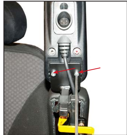
Flip up the armrest and remove the two screws that secure the joystick onto the joystick bracket.
