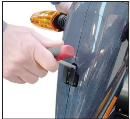
Adjusting the height of the handlebars.
