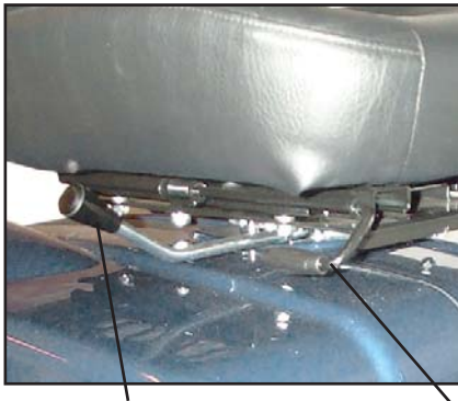
Release lever for seat rotation. Release lever for seat forward/back.
