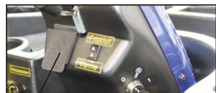
Connect the charging plug to the 3-pin socket on the steering column. The charging socket is located under the protective cover.
