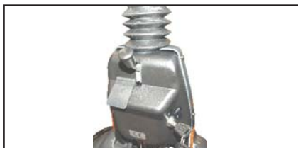
Connect the charging plug to the 3-pin socket on the steering column. The charging socket is located under the protective cover.
