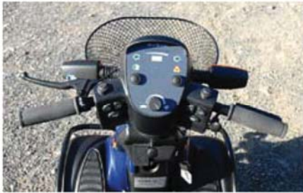
Well set-out: wipers and horn can be operated on both sides, but on the standard model the acceleration and brakes can unfortunately so far only be operated on one side.
